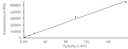
**Fig. 4:** Linear fit Nephelometric vs. Turbidimetric High NTUs. Formazin of 9 different concentrations were read using a HACH® 2100N turbidimeter and subsequently using the NEPHELOstar <sup>Plus</sup>. The two highest NTU standards (779 and 971 NTU) were eliminated due to a lack of linear correlation. However, it is of potential interest that including the higher standards in the data set resulted in a regression that correlates with a 4-parameter fit ( $r^2 = 0.9998$ ) [not shown].
