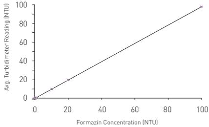
**Fig. 2:** Linear fit for Turbidimetric LOD. Formazin of 8 different concentrations were read using a HACH® 2100N turbidimeter and exhibit a linear fit ( $r^2 = 0.9999$ ).
