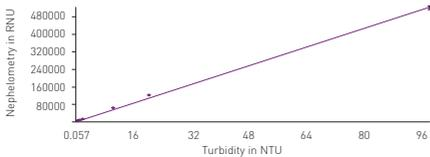
**Fig. 3:** Linear fit of Nephelometric vs. Turbidimetric Data Formazin of 8 different concentrations were read using a HACH® 2100N turbidimeter and subsequently using the NEPHELOstar <sup>Plus</sup>. The results indicate a good linear fit to over 90 NTU ( $r^2 = 0.999$ ).
