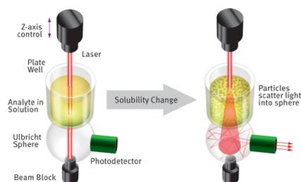
**Fig. 1: NEPHELOstar Plus detection principle.** A) Samples with little to no particles do not exhibit light scattering, light does not reach the photodetector and RNUs are low. B) Particles in solution scatter light, which reaches the photodetector and RNUs are higher.
