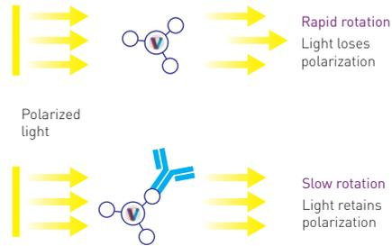
**Fig. 2:** Assay Principle: The assay applies fluorescence polarisation to quantify IgG. Concentration is measured by detection of changes in light polarisation caused by molecule rotation. Small, unbound molecules rotate rapidly in solution, while large, bound molecules rotate slowly.
