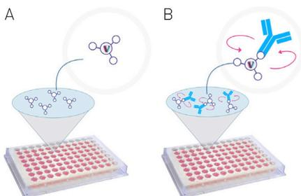
**Fig. 1:** Assay schematic of Valita™TITER assay for IgG quantification using fluorescence polarization: Each well of the 96-well Valita™TITER plate is pre-coated with a fluorescently labelled IgG binding peptide, protein G (A). IgG sample binds to the peptide and binding is measured via fluorescence polarization and rotational diffusion (B).
